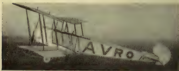
AVRO TRACTOR BIPLANE ( Flight ) 30 to 83 miles per hour
